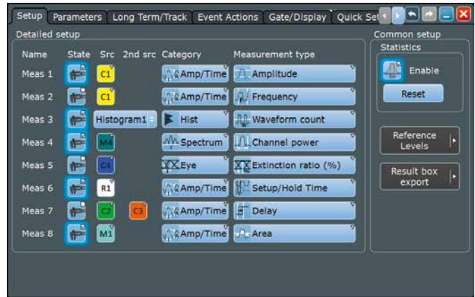
Fig. 4: In the R&S® RTE oscilloscopes, up to eight automatic measurements can be configured and activated simultaneously.
