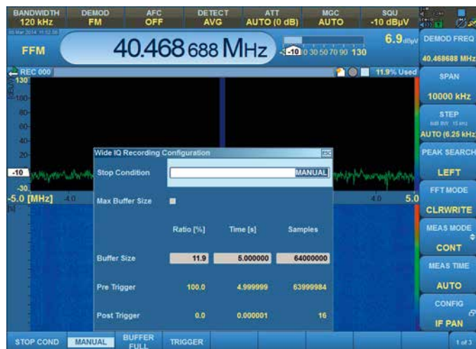
Fig. 3: In MANUAL mode, the user monitors the signals in the spectrum and stops recording at the right moment.
