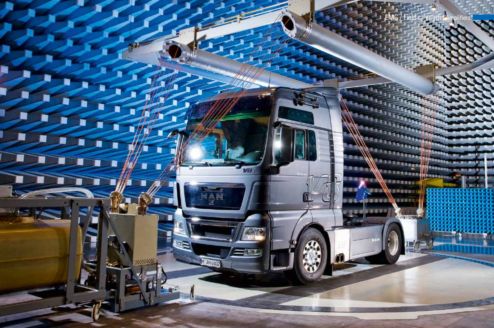
Fig. 1: High field strengths are required for EMS measurements on trucks, for example. The new R&S®BBL200 broadband amplifiers offer up to 10 kW RF power and generate the required field strengths in the frequency range from 9 kHz to 225 MHz.
