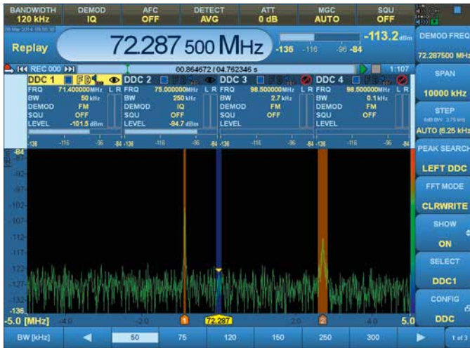
Fig. 5: Use of digital downconverters for replaying I/Q data.
