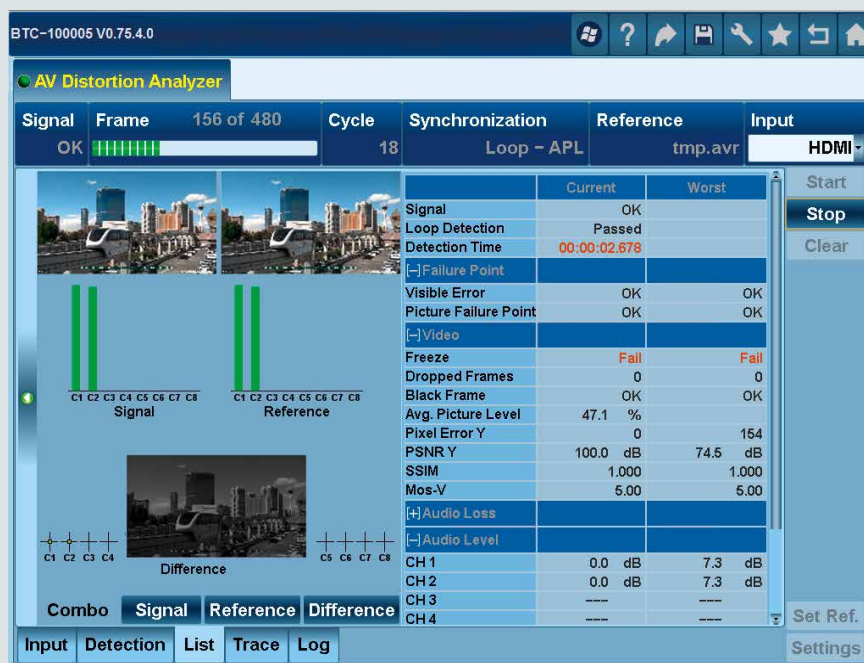
Fig. 2: The distortion analyzer of the R&S®BTC combines various picture quality parameters in a clear analysis screen.
